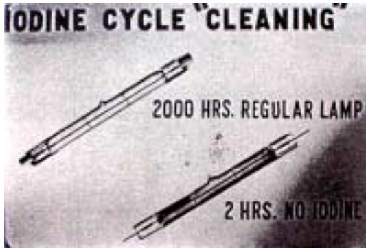
Figure 6: Original 500W tungsten-halogen incandescent lamp. (GE, 1959, [2])
